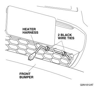
26. Attach the protective cap to the front bumper, and plug the heater harness connector into the protective cap.
