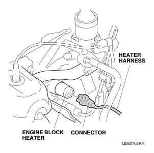
12. Secure the heater harness to the vehicle bracket with one wire tie at the white mark (point A).
