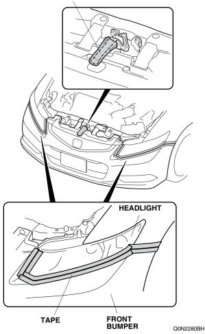
Remove the four self-tapping screws, ten short clips, and two long clips. Note the location of the long clips.
