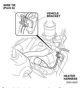
13. Route the heater harness as shown. Secure the heater harness to the fan shroud rib with one wire tie at the white mark (point B).
