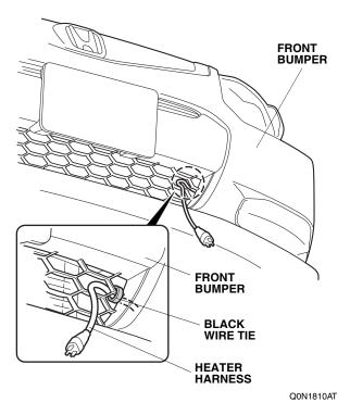
24. Route the heater harness inside the front bumper as shown.
