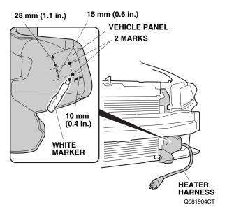
20. Using a pushpin, pierce the two marks you made into the vehicle panel at the location shown. While wearing eye protection, drill the two pierced marks with a 3 mm drill bit, then enlarge the holes with a 5 mm drill bit as shown. Remove any burrs.
