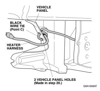
22. Route the heater harness through the front bumper as shown, then reinstall the front bumper with the help of an assistant.
