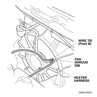
14. Route the heater harness along the top of the fan shroud.
