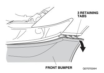
• On each side, release five retaining tabs.
