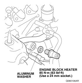
Plug the connector end of the heater harness into the engine block heater. Make sure the heater harness connector is fully seated in the engine block heater.
